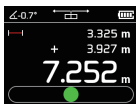
When measuring again, the instrument will automatically add the data and sum it up
